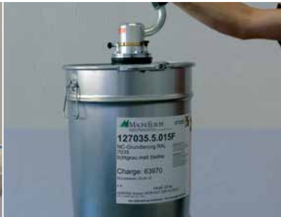
Single suction foot in bellows design
