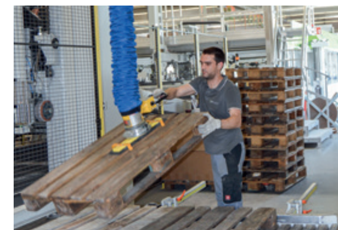
VacuPowerLift VPL-60KG With special suction gripper and centering unit for moving Euro pallets.
