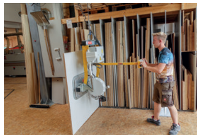
VacuPoro VP-90E-125KG Handling of wooden panels from an upright panel shelf system.
