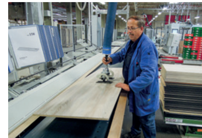
VacuQuickLift VQL-45KG Moving blockboards using a vacuum tube lifter.
