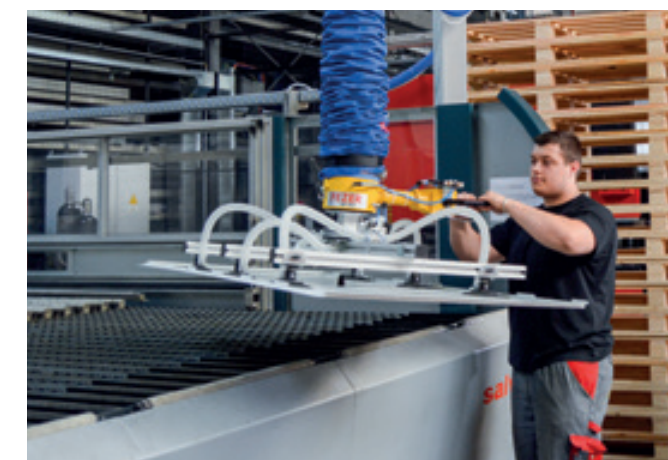
VacuPowerLift VPL-80KG Vacuum tube lifter for feeding sheet metal to a laser cutting system.
