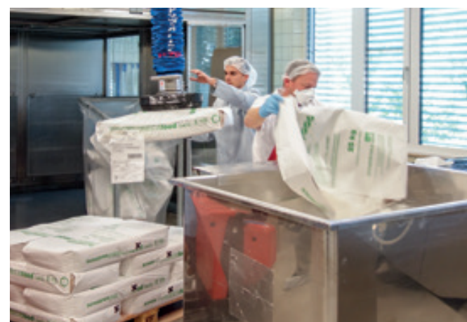
VacuPowerLift VPL-60KG Stainless steel vacuum tube lifter for handling single-layer paper bags.
