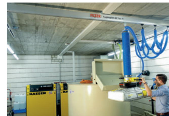
Aluminium overhead conveyor system HBS-EB-60KG with direct ceiling suspension and jacked-up single bridge for a low overall height.
