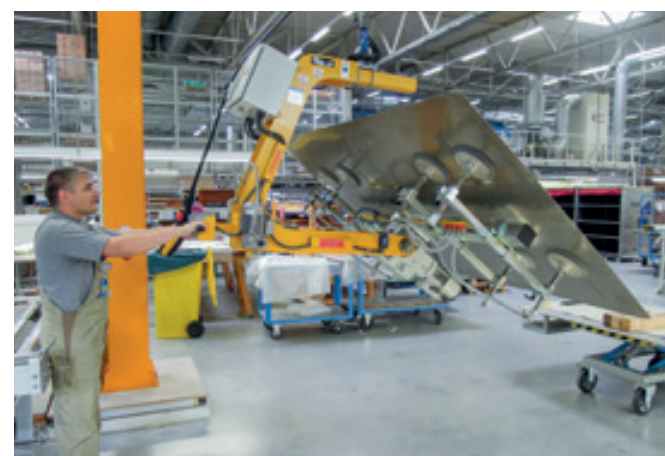
VacuBoy VB-180E-250KG 180° turning unit for sheet steel.
