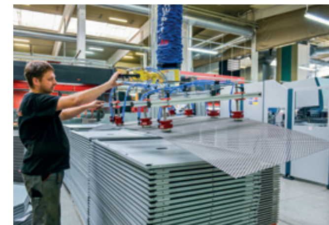
VacuPowerLift VPL-60KG Vacuum tube lifter with pneumatically controlled magnetic grippers for perforated sheets.
