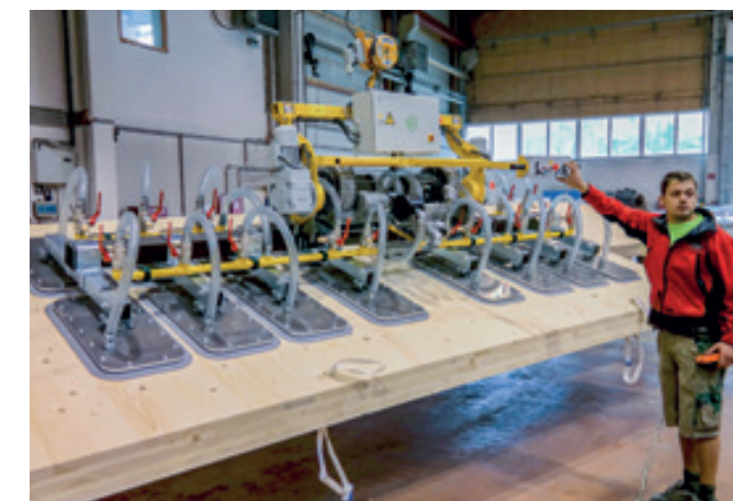
VacuPoro VP-90E-1500KG Vacuum lifter for swivelling solid wood panels 8,000 mm in length.
