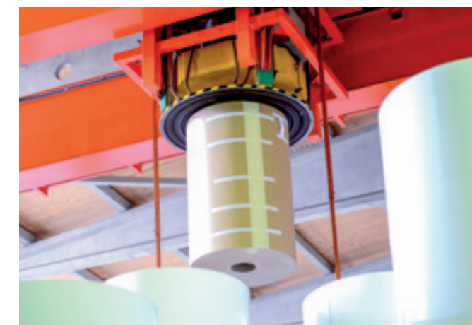
VacuCoilPaper VCP-5000KG-6SK cross beam on an automatic crane for picking paper rolls.
