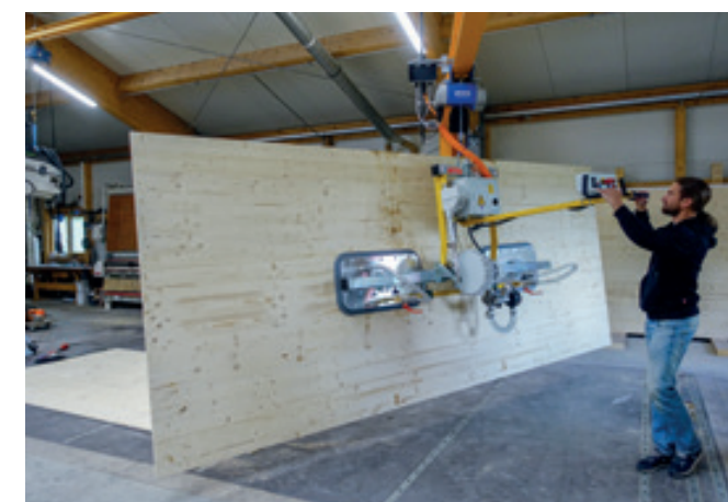
VacuPoro VP-90E-250KG Moving blockboards from an upright shelf system onto a panel saw.
