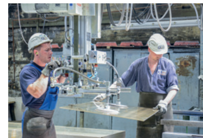
LiftFix LF-250KG Rigid lifting system with slewing ring for loading an edge press with copper sheets.
