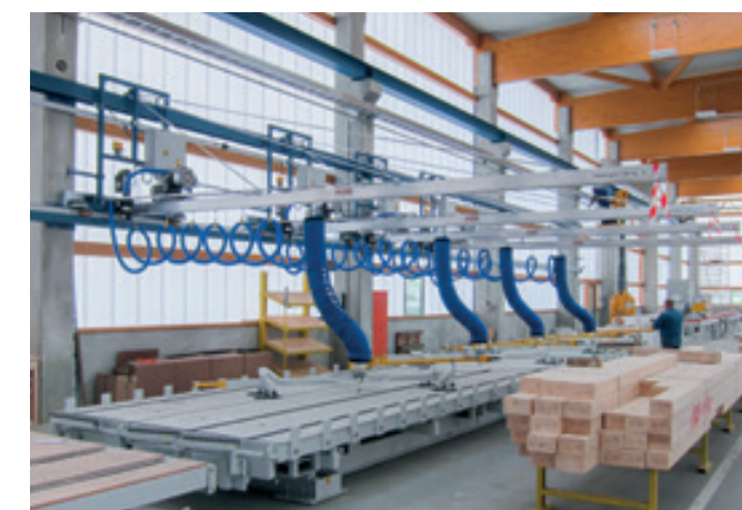
Aluminium overhead conveyor system HBS-4ALK-250KG Four jib crane systems, each with its own travel drive and moving blower for tube lifters.
