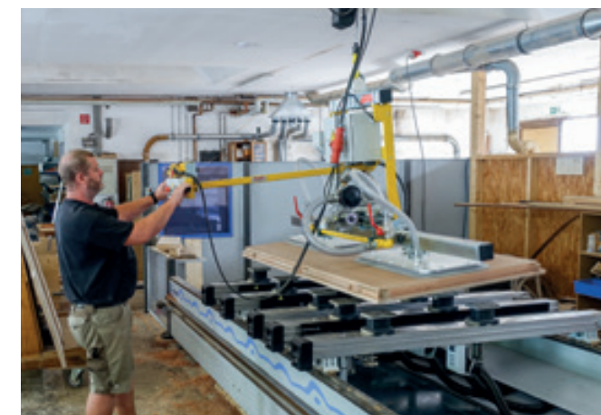
VacuPoro VP-90E-250KG Handling door elements on a CNC milling machine.
