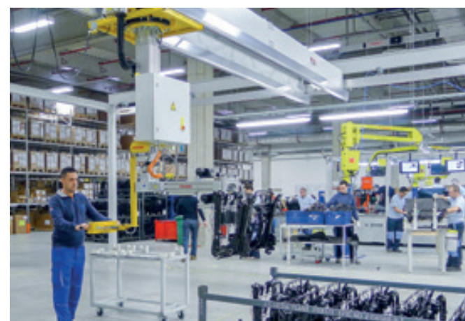
Aluminium overhead conveyor system HBS-DB-125KG With double bridge and rigid Liffix lifting system for moving seat frames.
