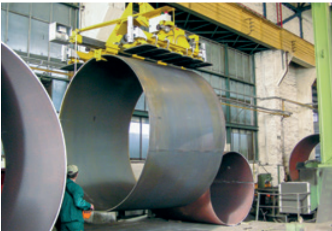
Vacuum Lifting Device VLM-6000KG Combination cross beam for handling sheet metal and pipes using vacuum and clamp technology.
