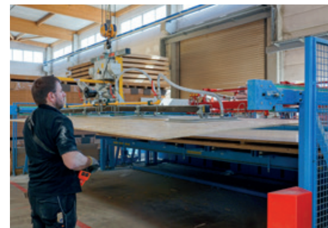
VacuPoro VP-90E-500KG Swivel-action lifting unit for loading a CNC woodworking system.
