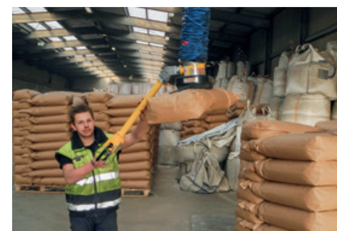
VacuPowerLift VPL-60KG Vacuum hose lifter for moving paper bags.
