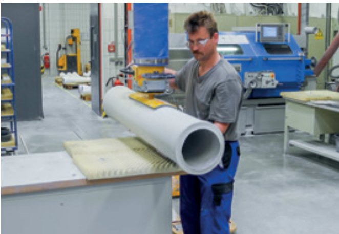
VacuPowerLift VPL-80KG Tube lifter with special gripper for moving concrete pipes.
