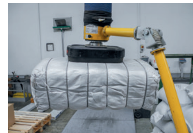
VacuPowerLift VPL-60KG Handling of plastic bags strapped with ropes.
