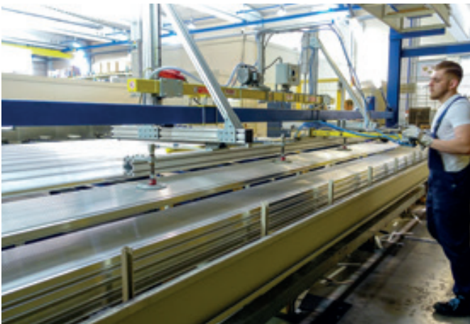
LiftFix LF-125KG Rigid lifting system with pneumatic stroke for feeding aluminium bars to a saw.
